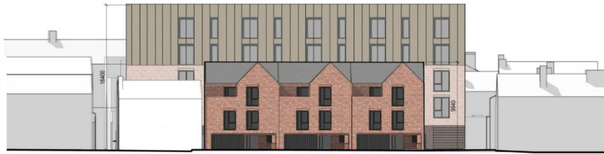
Elevational drawing of Allanson Street elevation showing proposed townhouses in the foreground and proposed apartment block beyond.
